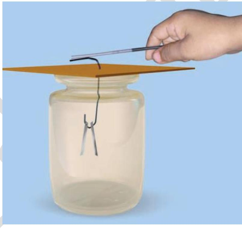
It is a device which is used to detect the charged on any object. Its working principle is like charges repel while unlike charges attract each other.
