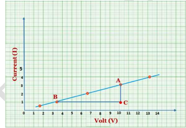
As we know the value of resistance is given by slope of the graph, so we consider two points A and B on the slope. From the graph, Now, BC = 10.2 V - 3.4 V = 6.8 VAC = 3 - 1 = 2 ampere Slope = 1/R = AC / BC = 2 / 6.8 = 1/3.4
