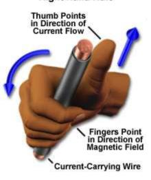
**Right hand thumb rule** states that if we hold the current carrying wire in the right hand and if the thumb points towards the current, the direction in which the fingers encircle gives the direction of Magnetic field.
