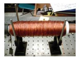
The magnetic field inside the solenoid is more but less outside it. Magnetic field inside solenoid is uniform i.e. same everywhere.
