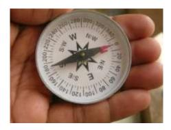
It is an instrument consisting of base and a needle. The needle has north and south tip whose north tip is painted red (generally). The needle gets deflected when close to magnet and it gives the direction of Magnetic field.
