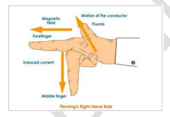
Similar to Flemings left hand rule, here we arrange our fore finger, centre finger and thumb of our right hand such that fore finger is in the direction of magnetic field, thumb is in the direction of motion, then centre finger would give the direction of current.
