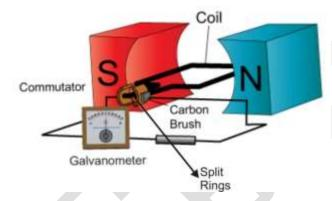
**Note:** The only difference between an AC and a DC generator is in the way the two ends of generator coil are linked to the outer circuit.
